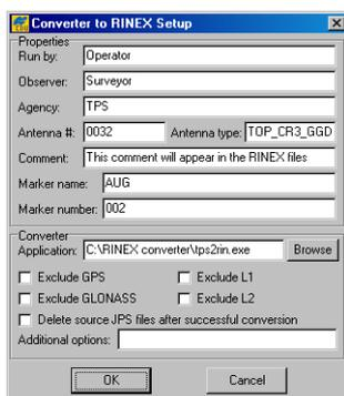
**Figure 3-19. Converter to RINEX Setup Window**
