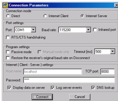
**Figure 1-12. Internet Server Connection Parameters**
