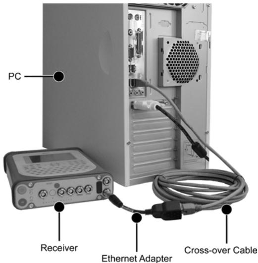
Figure 1-8. Direct Ethernet Connection – Hardware Setup
