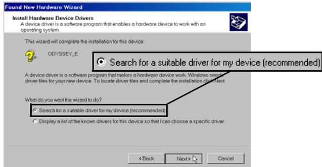
Figure 2-9. Windows 2000 – Install Hardware Device Drivers
